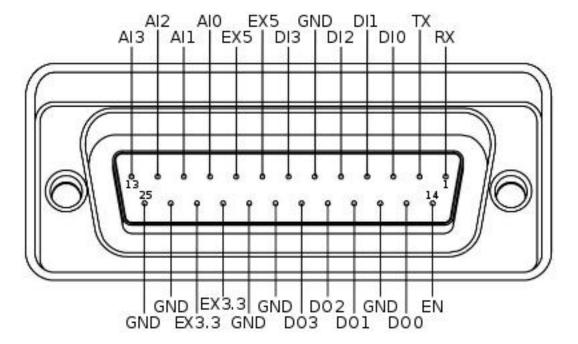
• RX/TX : Serial data (voltage level is 3.3V)
